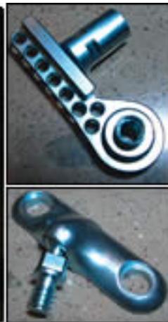
The titanium components of this assembled orthotic device are visible in this photo. The smaller photos show two of the individual machined parts from this assembly.
